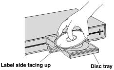
Place the disc on the disc tray with the label side facing up. Since disc size changes depending on the disc to be played back, be sure to correctly align the disc with the grooves for its size. If the disc is not in its groove, it may be scratched or otherwise damaged. To insert an 8 cm disc, place it according to the inner groove.
